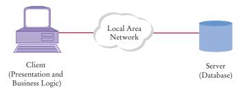
Figure 10 Two-Tier Client-Server Architecture
